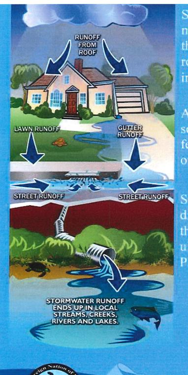
Stormwater is water from rain or melting snow that doesn't soak into the ground but instead flows over roofs, pavement, bare soil, and lawns into storm drains.
